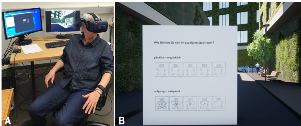
Figure 3. A study participant is wearing the VR headset and the EDA wristband on their left hand during the experiment (A). The SAM questionnaire is displayed in the virtual environment front of an urban scene stimulus with green façades (B).
