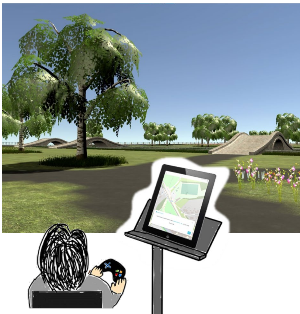
Figure 1. Playing GeoGami: The virtual world was projected on the wall. With the game controller, participants could move within the virtual world. They saw a map of the virtual world on the GeoGami game on the tablet. Participants received information about their tasks within the GeoGami game.
